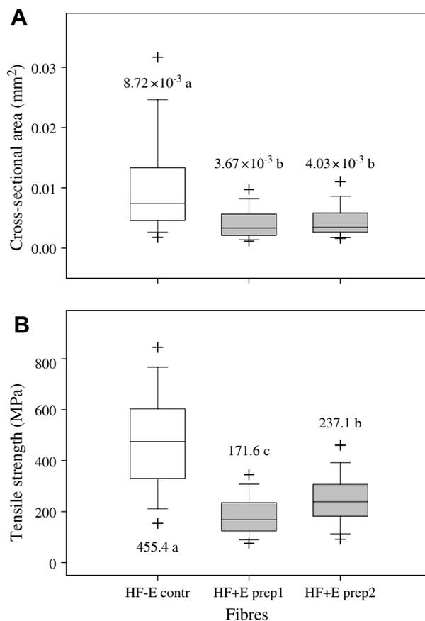
Fig. 1. Cross-sectional area (A) and tensile strength (B) of hemp fibres (HF) without (-E, contr) and with pectinase incubation (+E). Data for pectinase treated fibres were obtained from two independent preparations (prep1, prep2). Numerical data above boxes represent back-transformed arithmetic means. Different letters indicate significant difference of arithmetic means by ANOVA at  $P = 0.05$  (contr:  $n = 104$ ; prep1, prep2:  $n = 100$ ).
